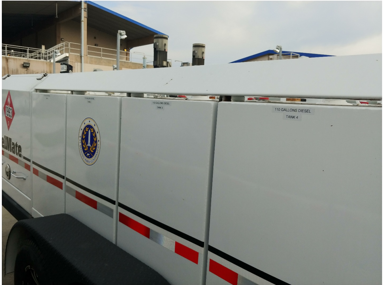
Storage capacity of diesel trailers, 8x110 gallons of storage each
